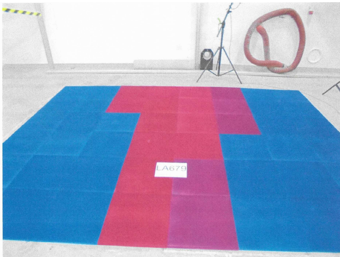
Pic. 1. Photograph of sample LA679, Fluffo Office flame retardant wall panels, in the reverberation chamber at the Laboratory of Vibro-acoustic Testing, Environmental CTO S.A.
