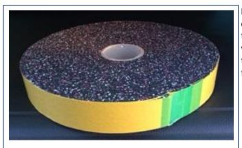
**Karma Isolation Strips** are acoustic isolating strips that are designed to sit beneath all types of wall partitions and on top of timber joists to provide a very simple and effective way to reduce structure borne noise. The strips can be tailored to fit all partition and joist widths creating solution for all eventualities.
