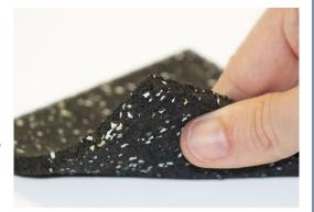
**Typical Applications** used in refurbishment projects, to isolate the partition/floating floor from the sub-base/joists below. In particular, houses, flats, offices, shops, hotels and nursing homes.
