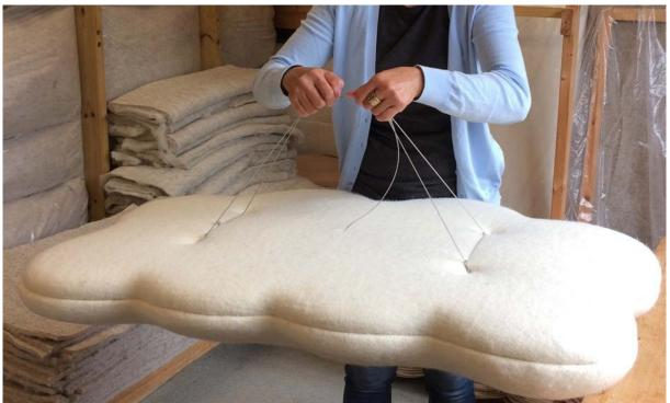
\*Never hold a cloud, or similar suspended absorber, at one end or allow them to be bent, as the internal structure can be broken and cannot be repaired.
