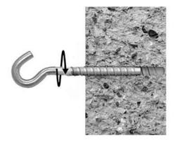
Insert Thunderbolt fixing and screw in clockwise direction.
