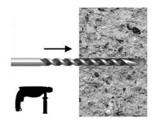
Using 6mm masonry drill make hole to 35mm depth.
