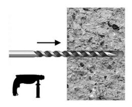
Using 6mm masonary drill hole to 50mm depth.
