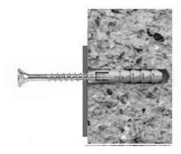
Hold plate in place and screw (M4 x 30mm) through into plugs.
