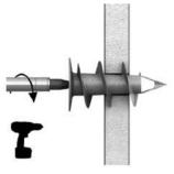
Using a PZ2 screwdriver, push fixing point firmly into the board until thread engages. Maintaining a firm pressure, screw in fixing until flush with the base material.
