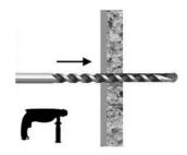
Drill through lath and plaster ceiling with 13mm masonry drill.
