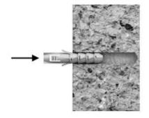
Insert plug and if needed tap lightly with hammer.
